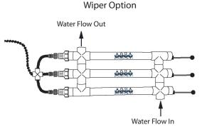
Plumb the water going in from the bottom and out through the top. This will help ensure the chamber stays full of water.
