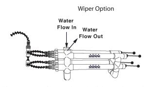
The above are suggestions, if these are inconvenient, either port can be used as the inlet or the outlet. In any installation the pump must be of a sufficient power to keep the chamber full of water so the seals around the wiper nut do not dry out.
