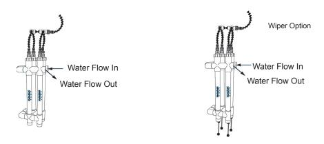
The above are suggestions, if these are inconvenient, either port can be used as the inlet or the outlet. For any installation it is important that the pump flow enough water to keep the UV chamber full; a partially filled chamber allows the seals to dry out including the wiper nut seal on wiper models.
