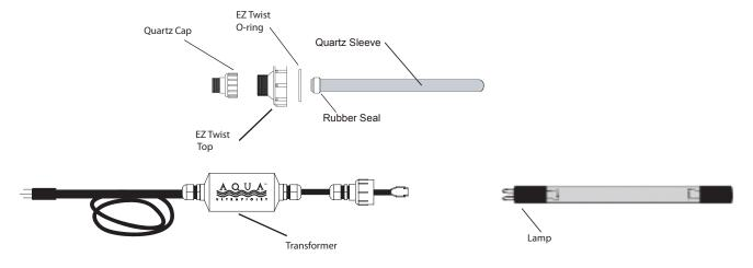
Option 2: If you are not flowing water through your system, use a winterizing cap, drain the unit completely and take the internal parts inside. If the unit is not completely drained, the water will freeze and crack the housing. This is not covered under warranty.
