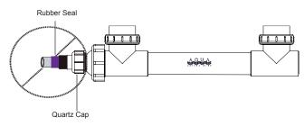
Incorrect: Quartz Sleeve Not Seated See Page 24 for Proper Quartz Sleeve installation
