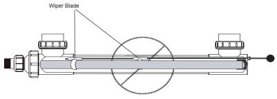
Lamp Dropped in Quartz Sleeve can Cause Breakage
