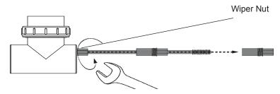
11. Pull the Wiper Rod from the large open end of the unit.
