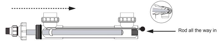
10. Screw on the EZ Twist top. Do not use a pipe wrench, pliers or any other tool on this unit. Tighten by hand only. Re-Install the lamp as shown on page 21, starting at #6.
